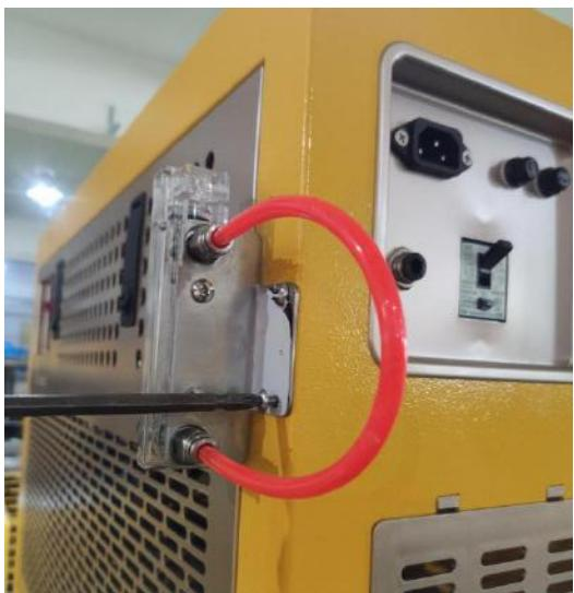
1、 Fix the flow meter on the machine using screws, and transfer the pipe of bottom interface to the machine.
