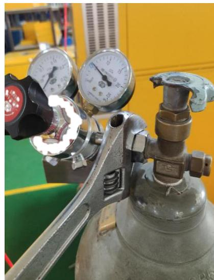
3. Connect the two ends of the red pipe to the interface below the flow meter and the pressure reducing valve.
