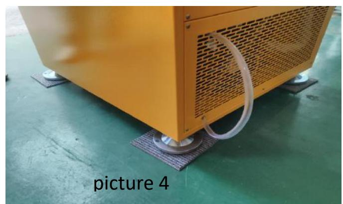
1. There are two screws, the lower one is used to adjust the height, the upper one is used to fix. (picture 3)
