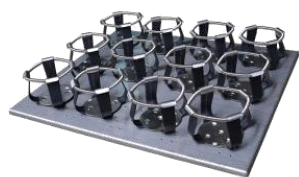
Universal platform with s.s. clamps
