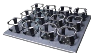
Universal platform with s.s. clamps
