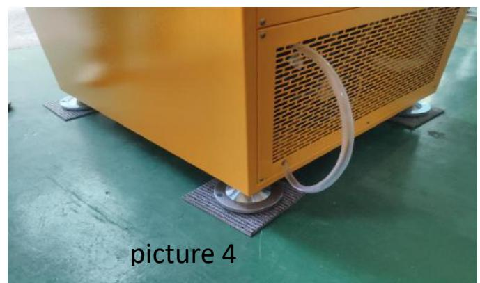
1. There are two screws, the lower one is used to adjust the height, the upper one is used to fix. (picture 3)
