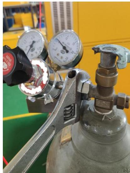
3. Connect the two ends of the red pipe to the interface below the flow meter and the pressure reducing valve.
