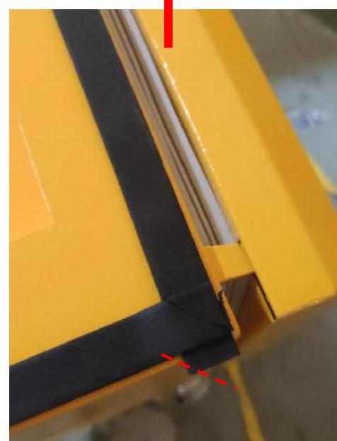
2. Use a utility knife to cut out a rectangle and expose the screw holes to prepare for subsequent stacking installation.
