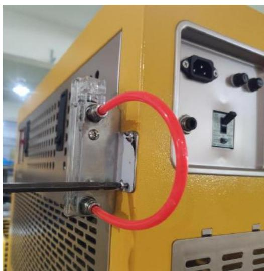
1. Fix the flow meter on the machine using screws, and transfer the pipe of bottom interface to the machine.
