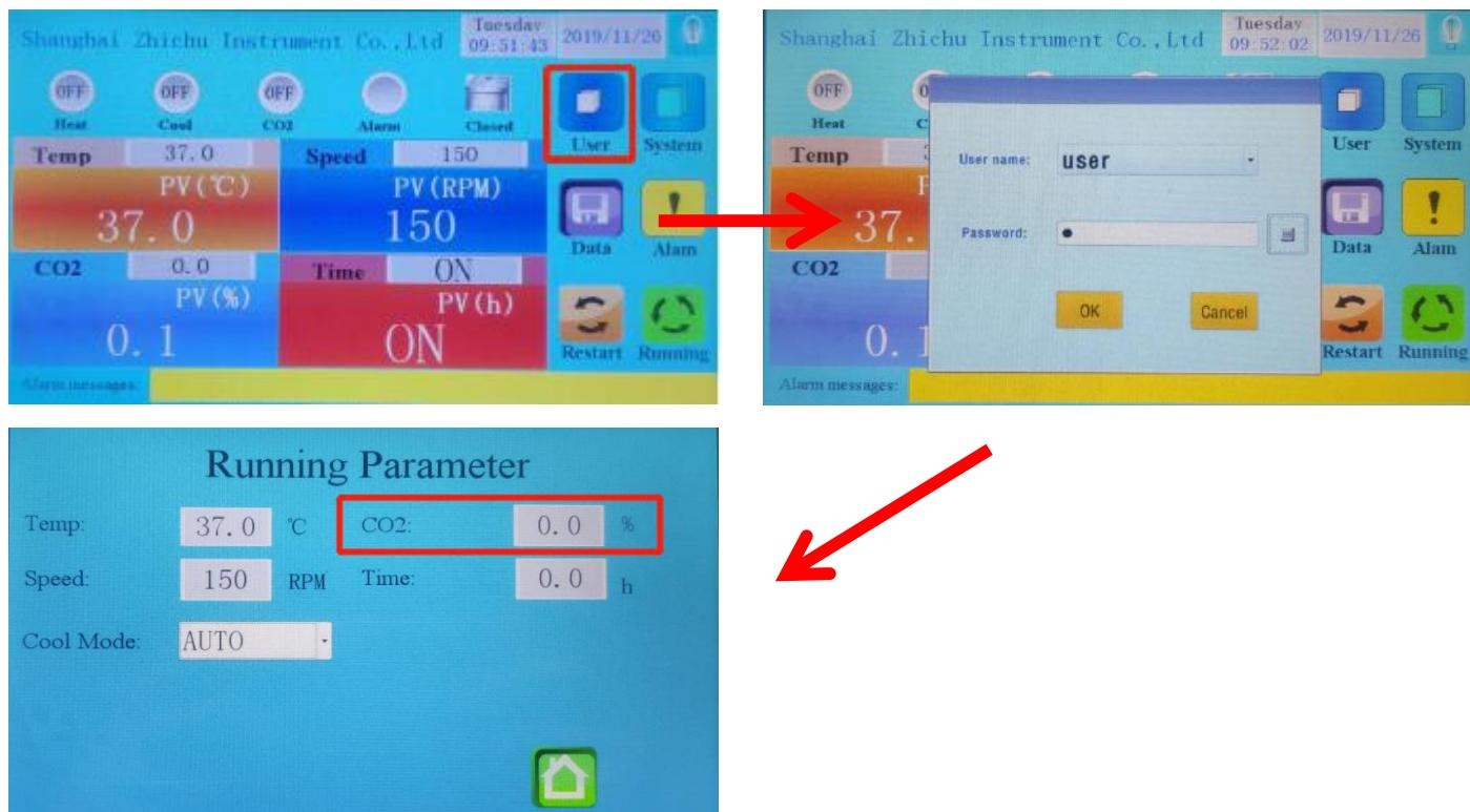
6. Click “System parameters”, and select“System” and enter password“12”, then make sure“CO2 function”is open.
